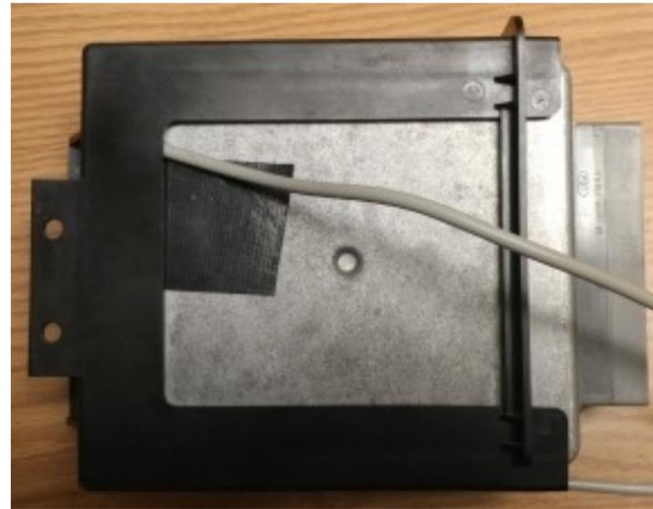
Be sure the box holding the computer in place does not bind the chip causing it to tilt and lose connection. Return the ECM to its location and re-connect the wiring harness and 2 bolts in box. Reconnect Batteries.
