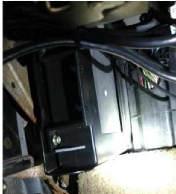
Once you have the ECM removed, on the opposite end of the wiring harness plug is a small plastic or metal cover. Remove this cover gently. Inside this J3 port is a circuit board with double-sided contacts that must be cleaned of conformal coating. J3 Port contacts must be cleaned thoroughly, or the chip will not make proper contact with the ECM.
