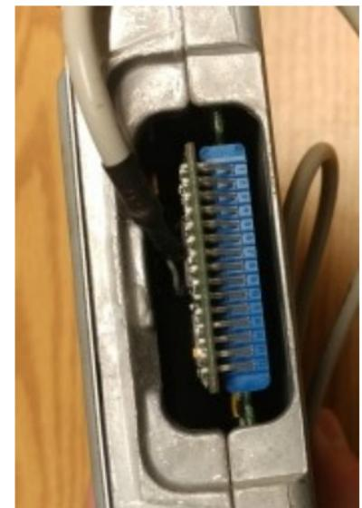
The proper orientation of the chip is with the circuit board of the chip and the switch cable on the larger side of the J3 port opening.
