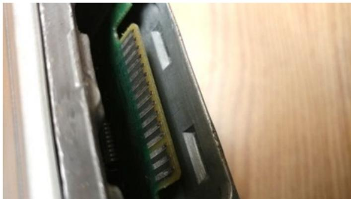
Scrub off the coating using the Scotch-Brite pad provided or a fine sandpaper. The contacts should start to become shiny and metallic copper color. Scrub only until you begin to see a hint of copper. Wipe off any remaining coating with rubbing alcohol or lacquer thinner on a paper towel.
