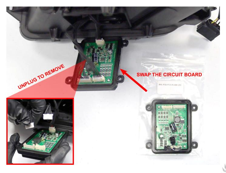
Plug the wires to the new circuit board for the swap.
