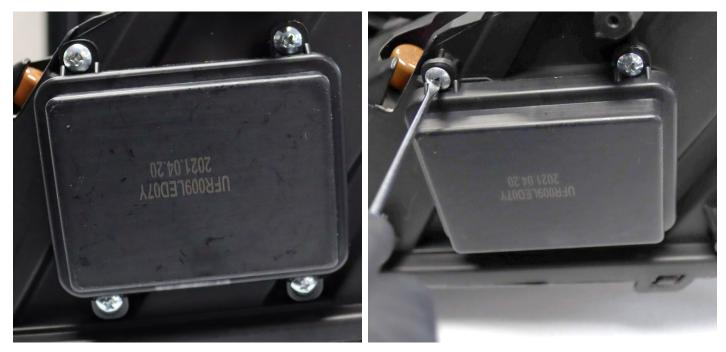
Unplug the wires to remove the factory circuit board and lets get ready for swap the optional circuit board.
