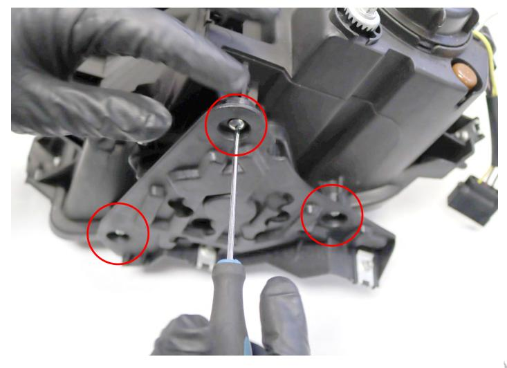
Once the mounting bracket is removed, you will have access to circuit board. Please unscrew the (4) screws to open.
