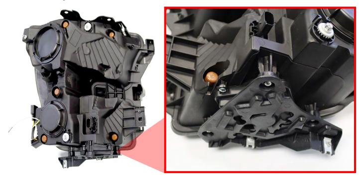
With a Phillip screwdriver unscrew the (3) screws from the mounting bracket.
