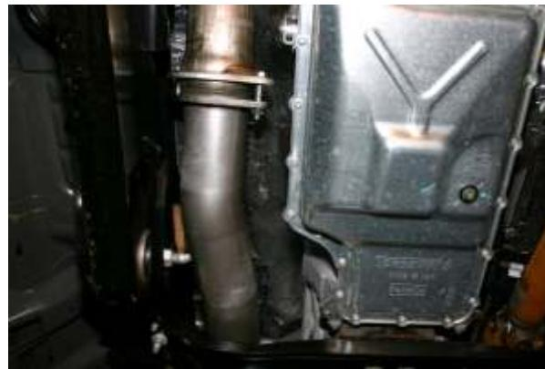
3. Next, install 31113NB pipe, extension pipe (Will need to be trimmed depending on wheelbase) and muffler delete pipe.
