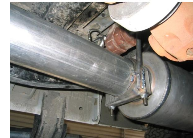
4. Install tailpipes placing metal hangers into OE rubber hangers. Place clamps on all connections.
