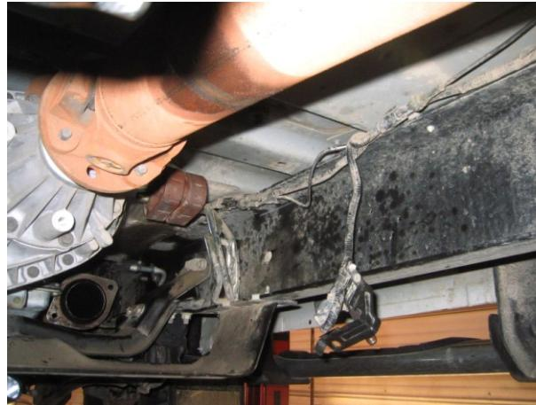
2. Install pipe with flange by placing welded metal hanger into OE rubber hanger and loosely tighten flanges together. Install 30813NB pipe and extension pipes depending on wheelbase. You may need to remove lines/sensors from OEM system or ty-strap them to the frame (follow tuner manufacturer's recommendations)
