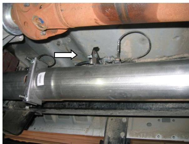
3. Install muffler by placing clamp hanger supplied over the inlet of muffler and place into OE rubber hanger.
