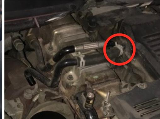
3. Install the Elbow (D) onto the CCV Filter (B) with the two #12 Hose Clamps (C). Tighten the hose clamp at the CCV Filter.
