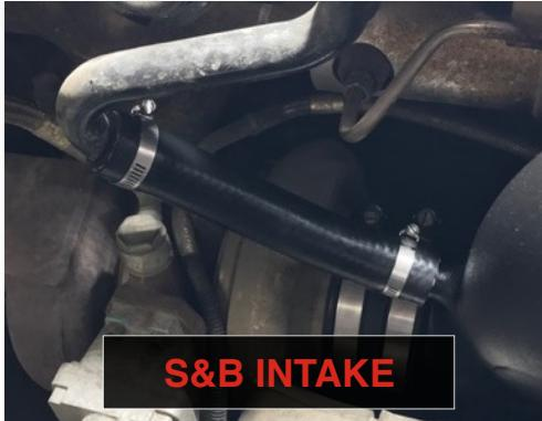
2. Remove the stock breather tube from the vehicle.
