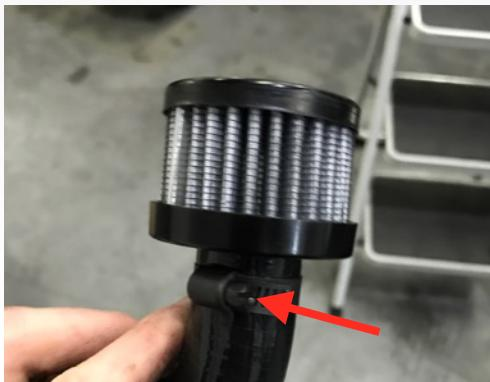
4. Install the CCV Breather assembly and tighten the #12 Hose Clamp (C).
