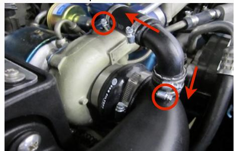
**18.** Completely loosen the clamp (E) around the Air filter base. Then carefully place the Air Filter (D) (base end first) inside the Air Box (P). Push the base of the filter over the Intake Tube (L) and tighten the hose clamp.
