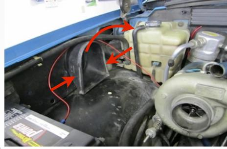
9. For those concerned about engine heat, insert the Air Box End Cap (Q) into the end of the Air Box (P). For those seeking additional air flow, set the Air Box End Cap aside. (See page 3 for more info)
