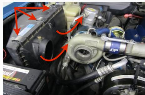
6. From under the wheel well, remove the 2 bolts mounting the air box.
