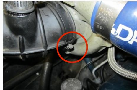
3. Loosen the hose clamp on the crankcase vent tube (CVT).
