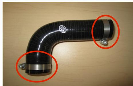
**17.** With the 2 #16 Hose Clamps in place, slip the longer hose end of the assembly onto the OE vent tube and then push the smaller hose end onto the intake tube. Fully tighten the all hose clamps.
