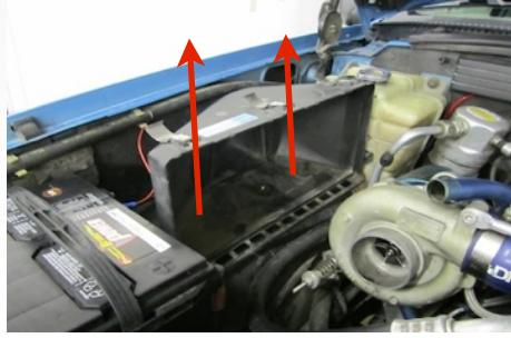
8. Remove the OE snorkel from the fender by pressing in the sides and popping it out towards the motor.
