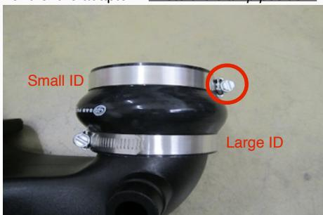
**13.** Install the intake tube assembly onto the turbo first and tighten the #52 Hose Clamp (G) at the turbo.
