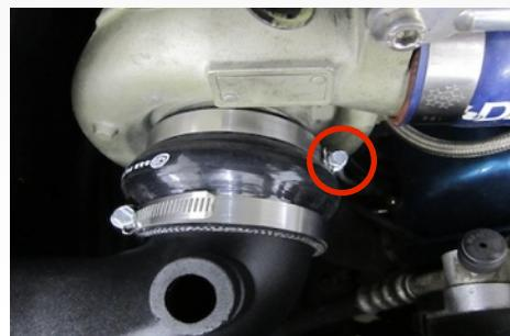
**14.** Hook the latch on the Intake Tube (L) to the bottom edge of the Air Box (P). Secure the tube to the box using the 2 supplied 3/8" Truss Screws (M).
