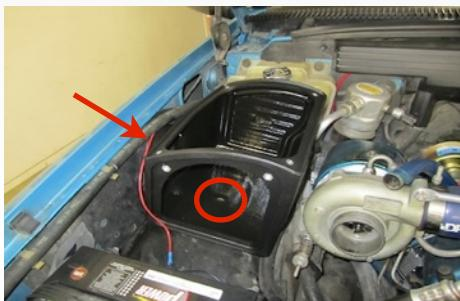
**11.** Loosely install the Air Box (P) to the wheel liner using the supplied 3/8" x 1.0" Button Head screw (F) and Fender Washer (O) on top and the 3/8" Nylock Nut (N) and Fender Washer in the wheel well.
