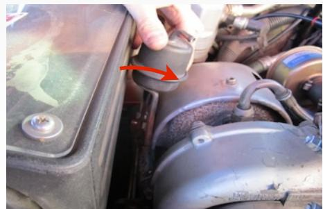
**12.** Install the Silicone Turbo Adapter (H) to the Intake Tube (L). Install the larger ID end on the tube using the #56 Hose clamp (I). Place the #52 Hose Clamp (G) on the smaller end of the adapter. \*Note the clamp position\*
