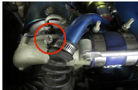
4. Loosen the clamp at the tube/ air box connection. Then remove the tube assembly from the truck.
