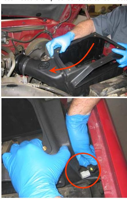
15. When the S&B air box is in place, secure using the OE nut and washer.
