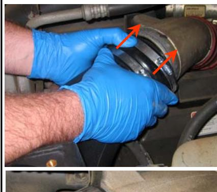
19. Install the S&B air filter (C) to the S&B air box adapter (H), secure the # 72 hose clamp.
