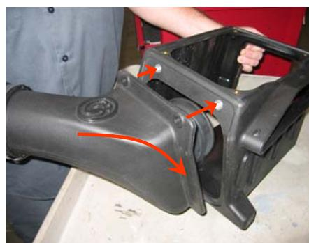
14. Place the S&B air box assembly in the vehicle. Before seating the grommets, reconnect the temp. sensor electrical connector.
