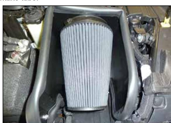
14. Install the K&N® air filter and secure with the provided hose clamp.
