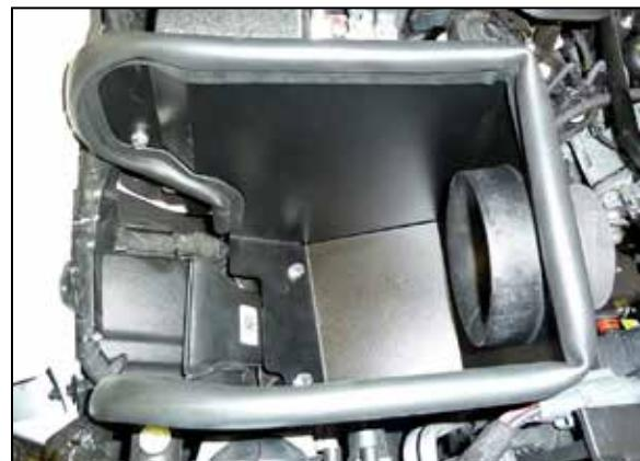
11. Install the heat shield assembly into the vehicle so that the mounting studs insert into the factory mounting grommets.
