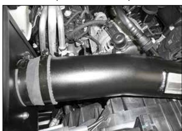
13. Connect the crank case vent line to the K&N® intake tube.
