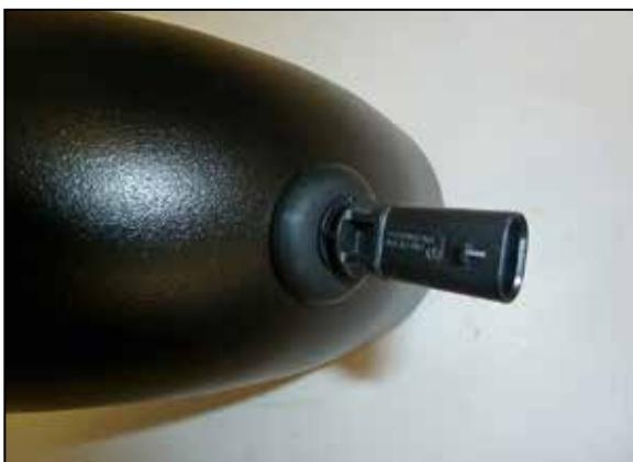
8. Install the provided grommet and factory temp sensor onto the K&N® intake tube.
