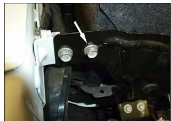
5. Remove the inner bolt that attaches fender bracket to the fender.
