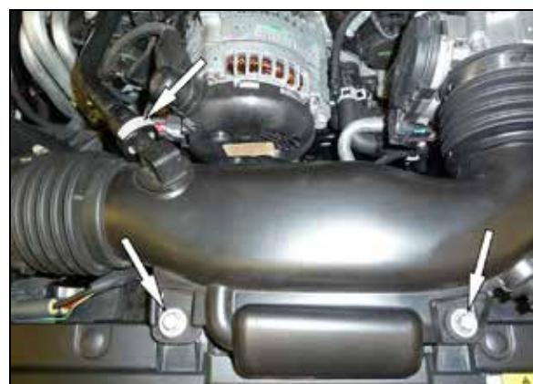
3. Remove the two bolts shown that secure the intake tube to the core support. Push the white locking tab for the crank case vent line down and then disconnect the crank case vent line from the intake tube.
