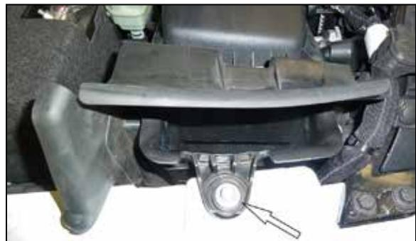
4. Remove the bolt shown that secures the fresh air intake duct to the fender, then lift and remove the complete intake system from the vehicle.
