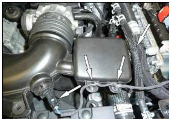
2. Disconnect the inlet air temperature sensor connection and unhook the wiring harness from the intake plenum. Unhook the coolant by-pass hose from the intake plenum and loosen the hose clamp that secures the tube to the throttle body.
