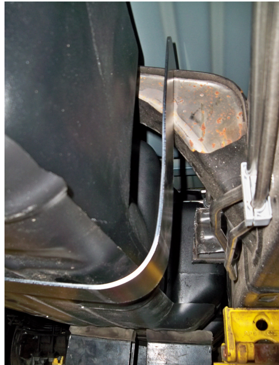
(Fig. 16) Hanger Bracket installed on frame cross-member. Since a TITAN Shield is used no bushing is installed.
