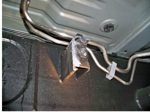
(Fig. 10) Jig bracket shown cut away leaving weldment holding fuel lines.
