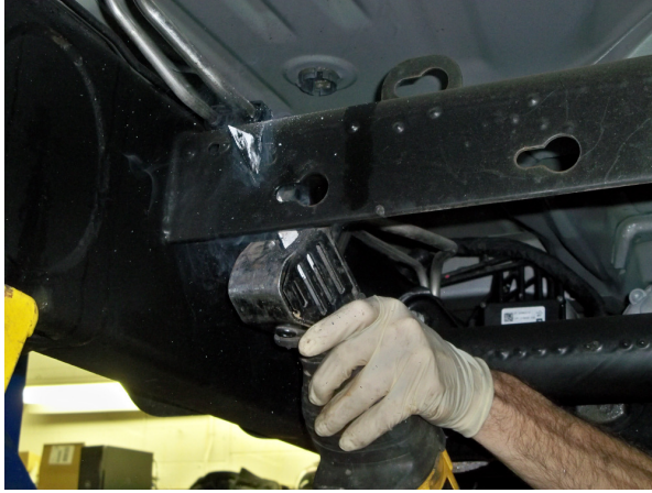
(Fig. 9) Cut jig bracket with saw or grinder.
