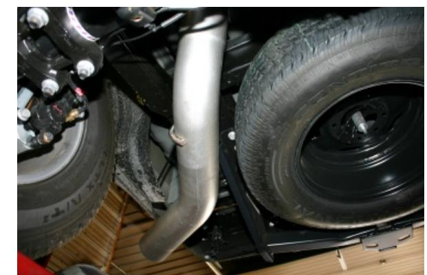
5. With the pipes mounted loosely, adjust the new Flo-Pro system for clearance and appearance. Evenly tighten all clamps starting with the front flange connection working your way to the back.
