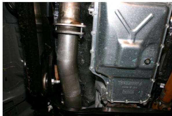
3. Next, install 31152NB pipe, extension pipe (for Crew Cab Long Box) and muffler. You can use a stand to support the muffler in place.
