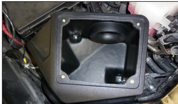
12. Install the K&N air filter housings onto the rubber mounted studs and then secure the housing with the provided hardware.
