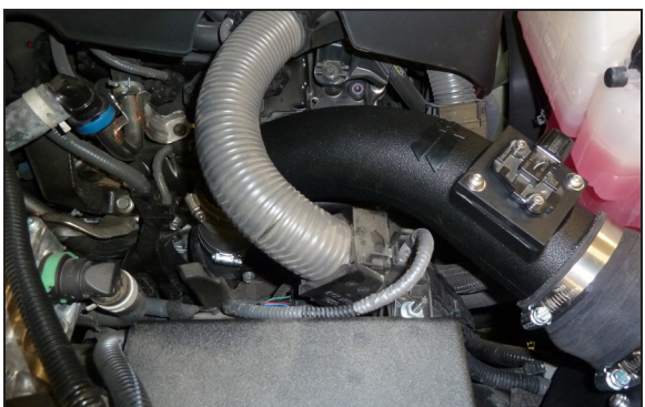
16. Apply four drops of the provide super glue to the lip of the MAF sensor grids then, install the mass air sensor grids into the K&N intake tubes as shown.
