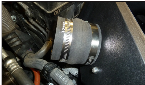
13. Install the provided hump couplers onto the filter adapters and secure with the provided hose clamps.
