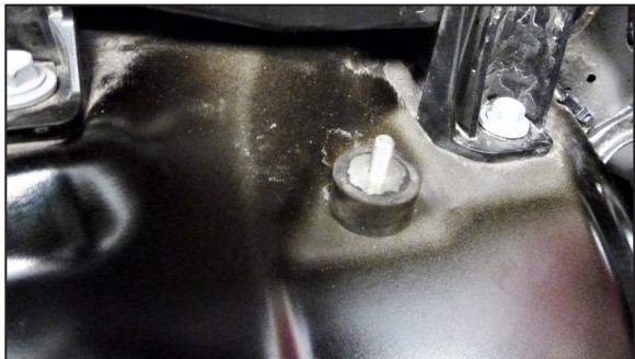
11. Install the provided rubber mounted studs into the rear most factory air box mounting stud locations.
