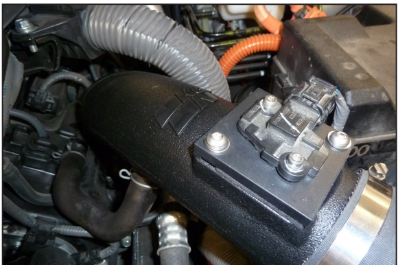
18. Connect the factory CCV hoses to the fittings installed into the K&N intake tubes. Reconnect the mass air sensor electrical connections.
