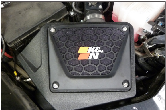
19. Install the K&N air filters onto the filter adapters and secure with the provided hose clamps.
