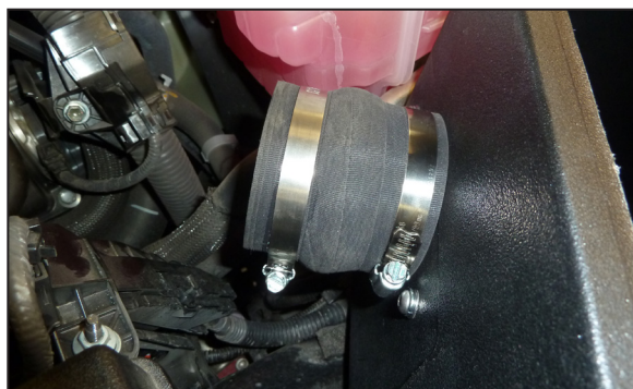
12. Install the K&N air filter housings onto the rubber mounted studs and then secure the housing with the provided hardware.
