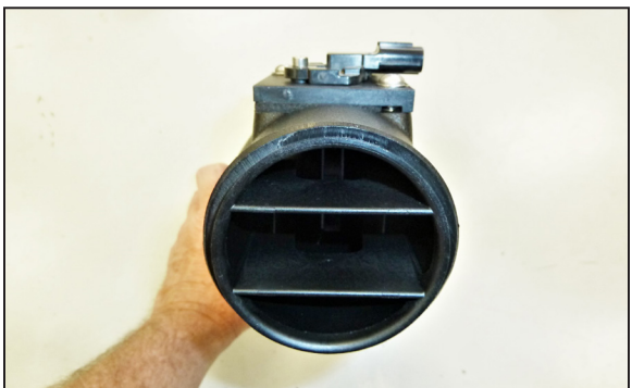
16. Apply four drops of the provide super glue to the lip of the MAF sensor grids then, install the mass air sensor grids into the K&N intake tubes as shown.
