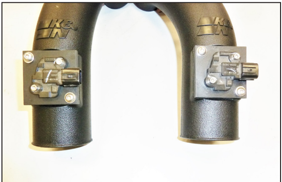
15. Using the provided adapter plates and gaskets, install the mass air sensors into the K&N intake tubes as shown.
