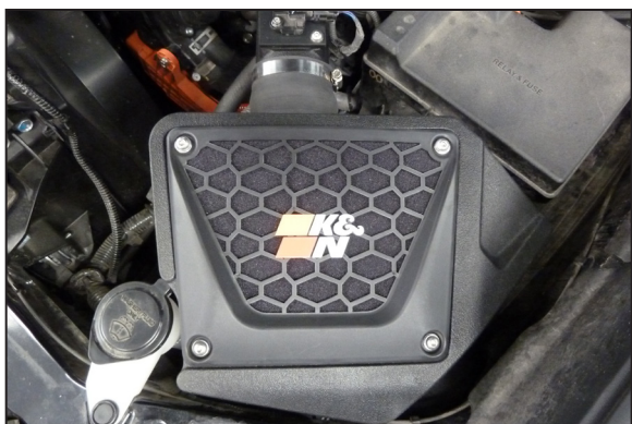
20. Assemble the two lid and foam lids and secure them to the air filter housings with the provided hardware.
