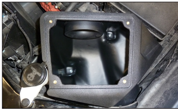
11. Install the provided rubber mounted studs into the rear most factory air box mounting stud locations.
