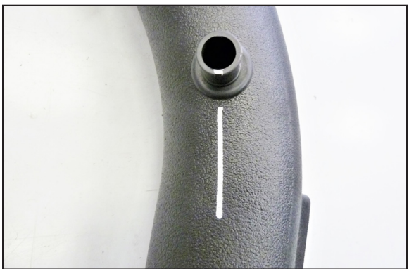
14. Install the CCV inserts into the K&N intake tubes with the provided grommets. Be sure the "notch" located on the bead of the insert is aligned as shown in the photos, the notch is to be towards the inlet end (towards the mass air sensor) of the tube.
