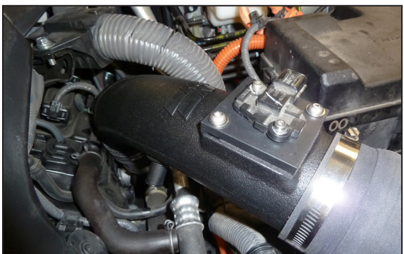
17. Install the K&N intake tubes into the couplers and adjust for best fit then secure with the provided hose clamps.
