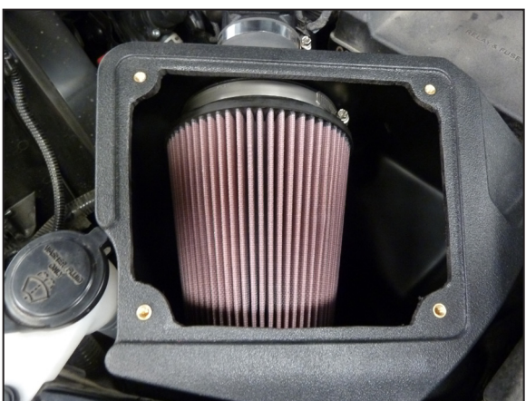
19. Install the K&N air filters onto the filter adapters and secure with the provided hose clamps.
