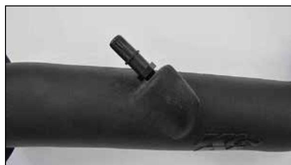
12. Install 1/4 NPT quick connect fitting onto the tube.
