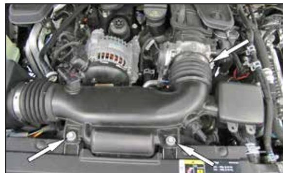
4. Remove the bolts that secure the factory tube to the fan shroud, then loosen hose clamp at throttle body.
