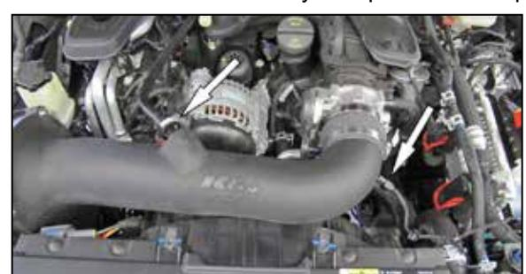
18. Reconnect the crank case vent line onto the quick connect fitting and reconnect the inlet temp sensor electrical connector onto the temp sensor.
