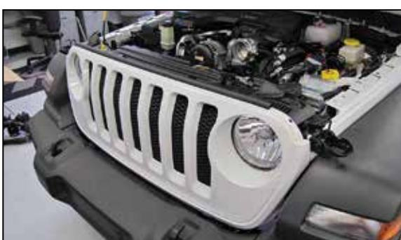
10. Reinstall the grill reengaging the lower clips one at a time then reinstall the six clips that hold the grill to the top of the core support.
