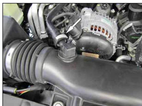
3. Disconnect the crank case vent line.
