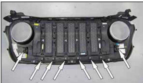
6a. Before removing grill note the location of the 8 clips that hold the lower part of the grill to the core support. Start at either side of the grill. Grasp the bottom part of the grill pulling firmly straight back dislodging the clips one at a time. Work your way across the grill until all clips have been dislodged and remove the grill.
