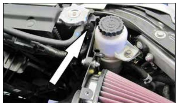
19. Install the heat shield bracket assembly onto the heat shield and radiator mount as shown. Secure the bracket with the factory bolt in step #9 and the hardware provided.
