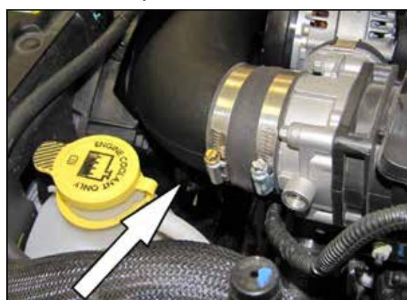
33. Reconnect the inlet air temperature sensor electrical connection.
