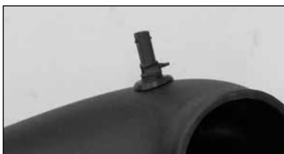
28. Install the provided grommet and factory inlet air temperature sensor into the K&N® intake tube as shown.
