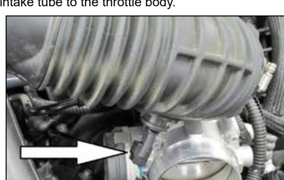
6. Lift up the intake tube, disconnect the inlet air temperature electrical connection then remove the intake tube from the vehicle.
