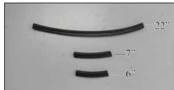
14. Cut the provided edge trim into three sections. One section is to be 6" long, one section is to be 7" long and the final section is to be 22" long.
