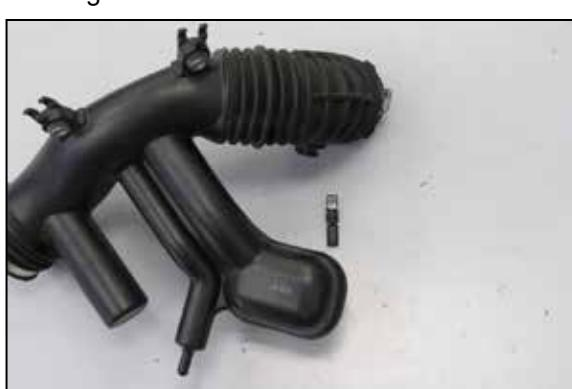
27. Remove the inlet air temperature sensor from the factory intake plenum as shown.
