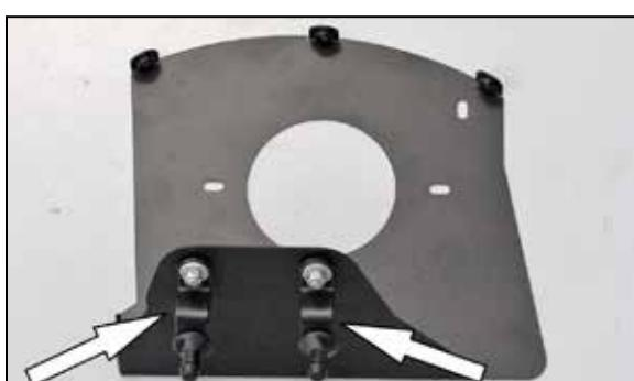
12. Install the two heat shield bracket assemblies onto the heat shield as shown.
