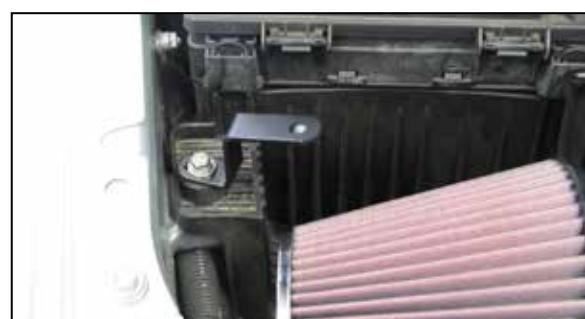
21. Install the provided bracket (083163) onto the rubber mounted stud using the provided hardware.
