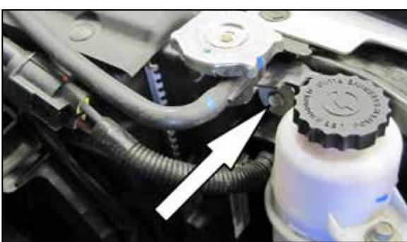
10. Remove the bolt shown that secures the radiator to the core support.
