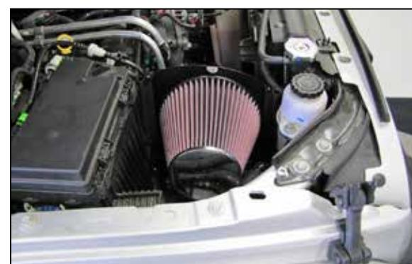
17. Install the K&N® air filter onto the filter adapter and secure with the provided hose clamp.
