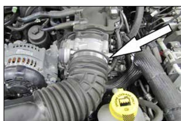
5. Loosen the hose clamp securing the factory intake tube to the throttle body.
