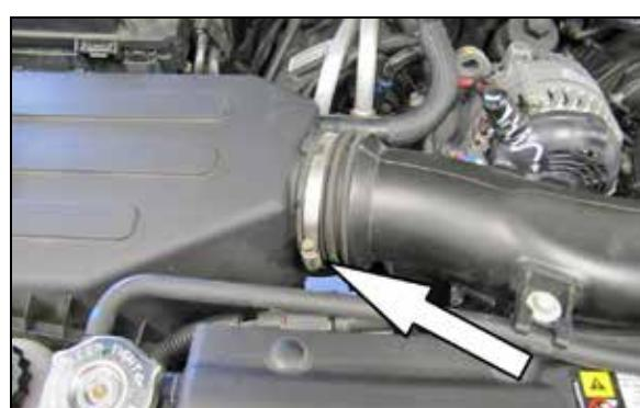
4. Loosen the hose clamp securing the factory intake tube to the air filter housing.
