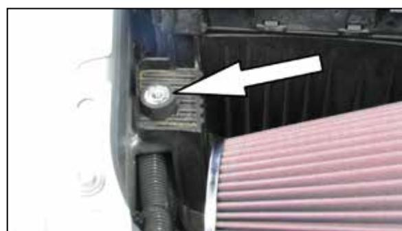
20. Install the rubber mounted stud into the into the air box mounting plate bolt location as shown.
