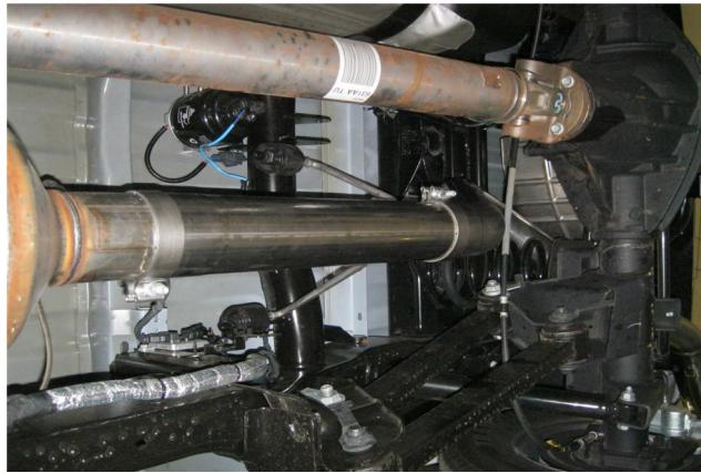
**Step 3.** The longer Inlet Pipe Extension will be needed for Long Bed applications only.
