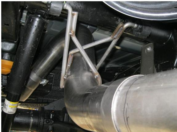
**Step 2.** Begin installation of the Magnaflow system by clamping the Inlet Pipe to the newly cut outlet of the DPF using a supplied 4.00" clamp and fitting the hangers in the rubber insulators (leave all clamps loose for final adjustment of the complete system).
