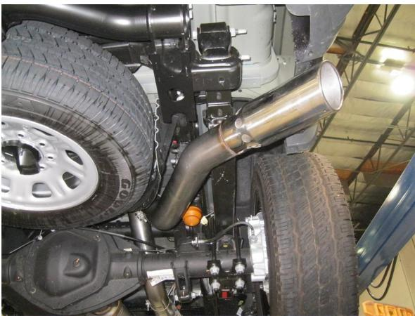
**Step 3.** Next Install the Tail Pipe Assembly in a similar fashion using the supplied 4.00" clamps and by fitting the welded hangers into the rubber insulators.
