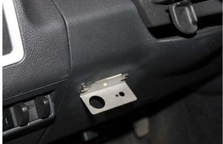
If mounting with double sided tape or Velcro, clean both surfaces with alcohol wipe. Alternatively to mount with a screw, bend the small locator tabs on the ends of the bracket downwards with needle nose pliers. Then drill a hole in the dashboard to accept the locator tabs. Install center screw to attach the assembly.
