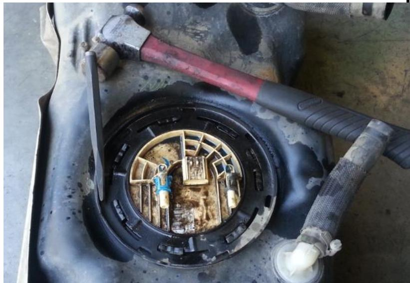
C. Using a pick or screwdriver, release the locking tabs that retain the fuel level sender. This will allow you to have more space to work.
