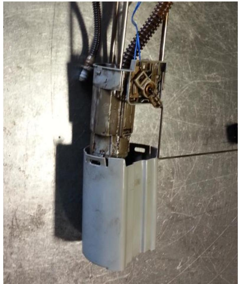
E. Pull the lower pickup bowl out of the assembly and cut the corrugated fuel line off the nipple using a razor blade
