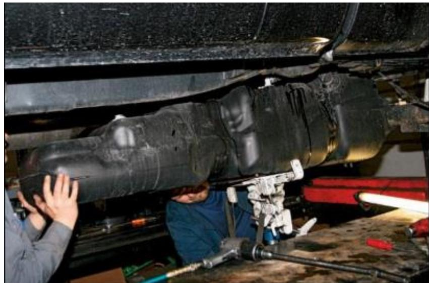
6. It is recommended to blow or wipe any debris around the perimeter of the fuel pickup away before pickup removal to avoid placing debris in the tank.
