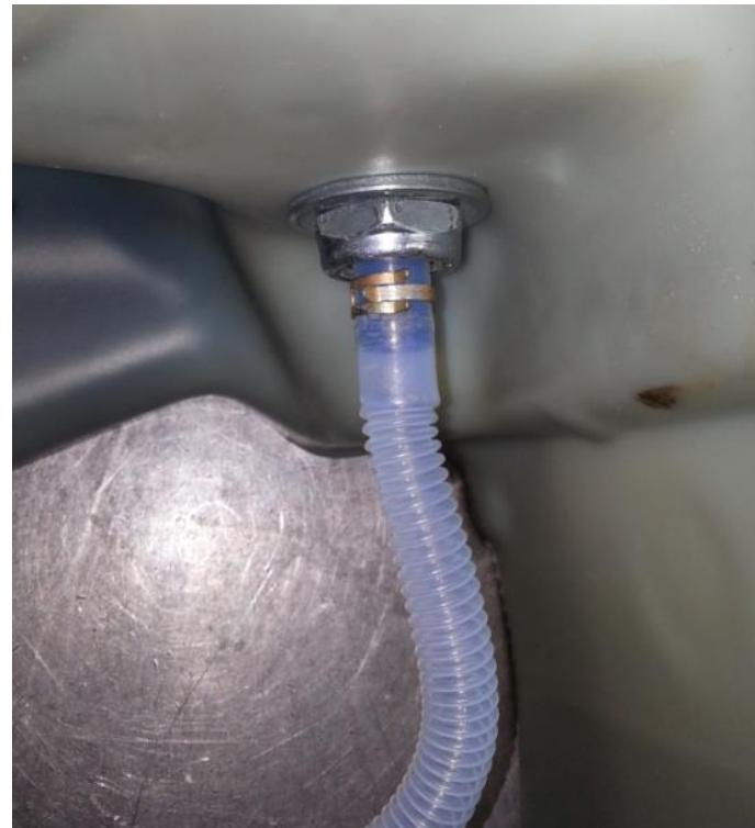
O. With the hose over the nipple, the fuel pickup assembly can be lowered back into place as shown. Slide another spring clamp over the hose then place the hose over the suction tube and secure with spring clamp.
