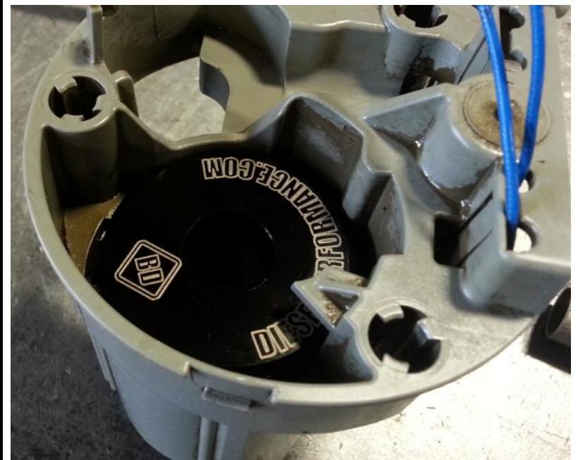
G. Drop the upper housing back into the lower bowl until the tabs click. Now, lower the machined pickup tube into the tube clamp until it rests on the bottom of the fuel bowl.
