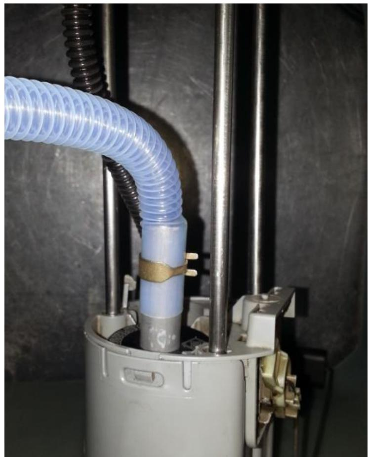
V. Reinstall the fuel pickup using the hammer and chisel or SST. Ensure the locking ring turns far enough to seat in the grooves. Push supplied rubber hose and 1/2" plug into the unused outlet line on fuel pickup. Install the spring clamp as shown.
