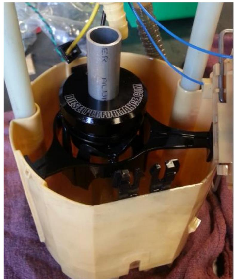
H. Now locate a flat area to place the bulkhead fitting. Ensure that there will be at least 1.5" of clearance above where the bulkhead is placed once the tank is re-installed.
