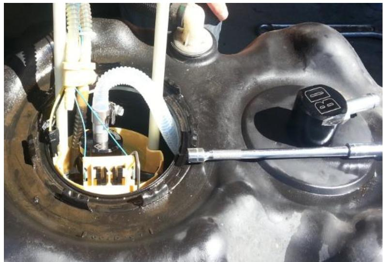
Q. Reinstall the fuel pickup using the hammer and chisel or SST. Ensure the locking ring turns far enough to seat in the grooves.
