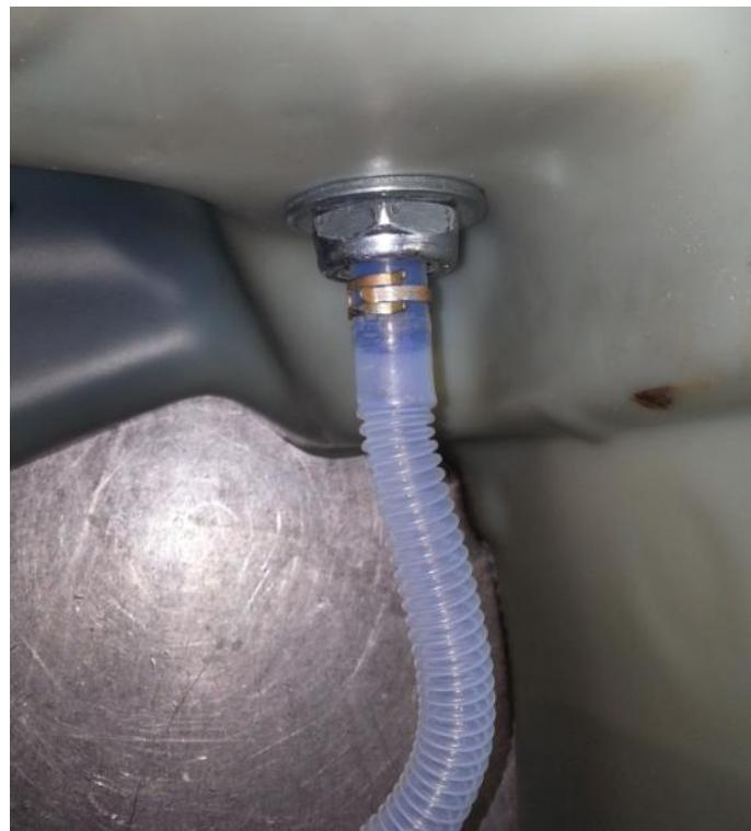
T. With the hose over the nipple, the fuel pickup assembly can be lowered back into place as shown. Slide another spring clamp over the hose then place the hose over the suction tube and secure with spring clamp.
