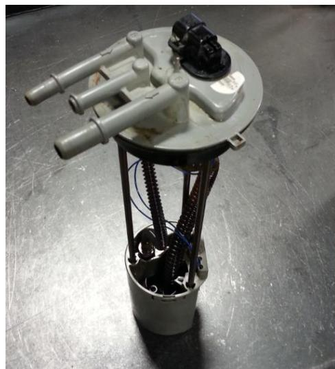
C. Using a screwdriver, release the fuel return nipple.
