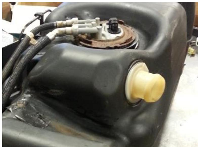
B. Remove the locking ring and lift the fuel pickup from the tank.
