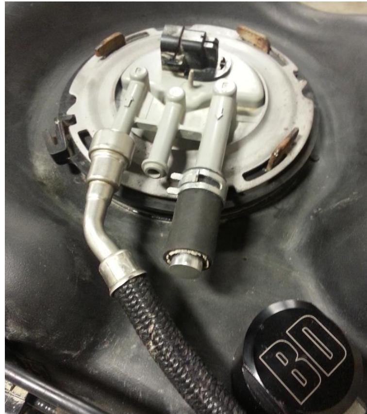
S. Connect the 1/2" fuel line to the bulkhead fitting and secure with the supplied hose clamp.
