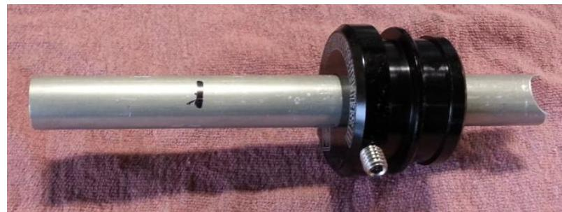
K. Again from the bottom, slide the pickup tube/clamp assembly up until the first click. Re-assemble the bowl and return line as shown.
