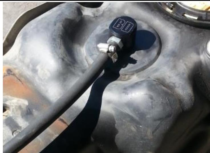
T. Lift the tank back into location and routing the new fuel line as necessary. Reconnect all vents, electrical connectors before lifting the tank back to its original location.
