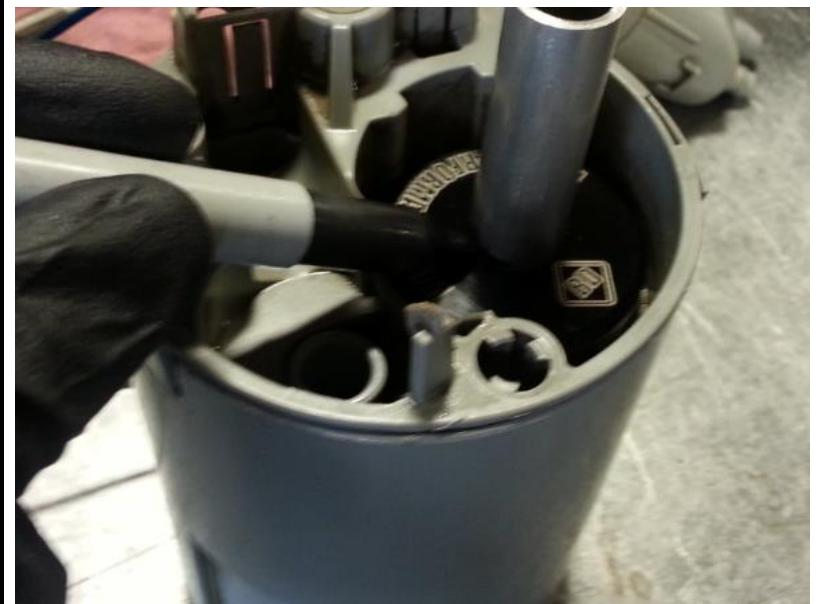
I. Using a long screwdriver, push the tabs in the housing and pull out the pickup clamp from the bottom. Use caution not to break the tabs.
