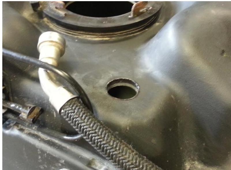
N. Check the hole for any burrs or edges that may cause a leak, deburr as necessary.
