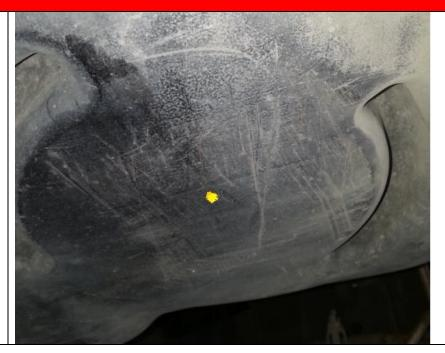
2. Now, create a 3" hole by drilling through the tank using the hole saw. If fuel remains in the tank, place a drain bucket below with a large enough capacity.
