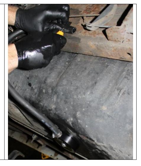
12. Now run your fuel line to the lift pump and cut to length. Secure the hose at both ends with the supplied gear hose clamps.
