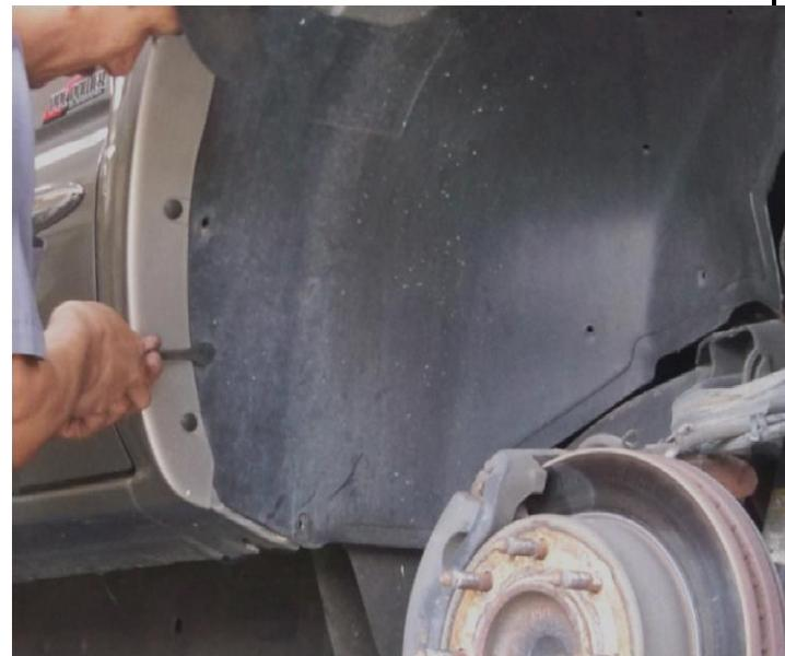
***Passenger side up-Pipe Removal and installation***
