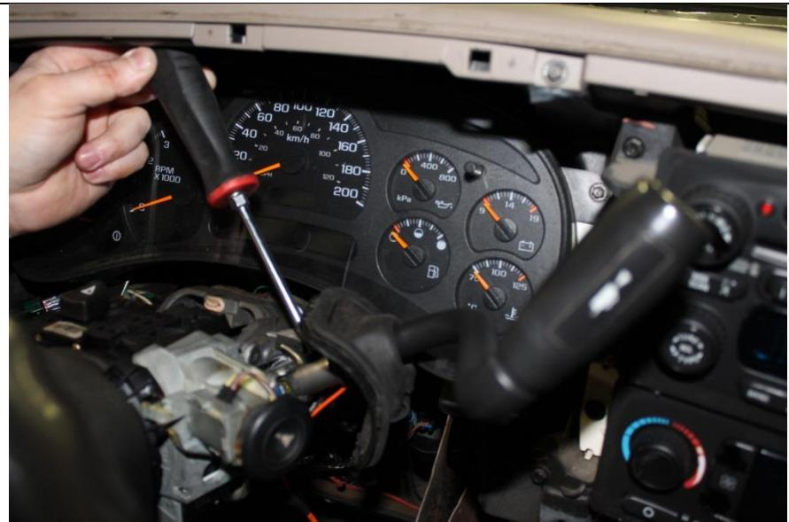
8. Reattach new lever with existing torx screw.
