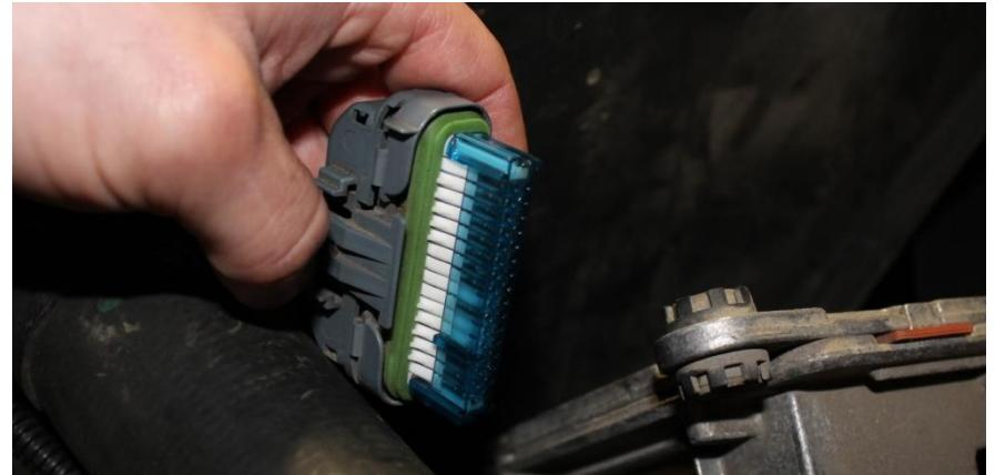
12. Connect the BD Tap Shifter wiring harness RED connector to the vehicles transmission control module.
