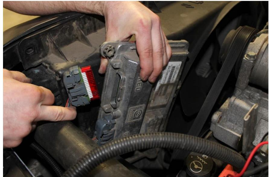
11. Remove the RED retainer on the vehicles transmission harness connector. Install the supplied BLUE retainer. Keep the removed RED key incase the module is ever removed.
