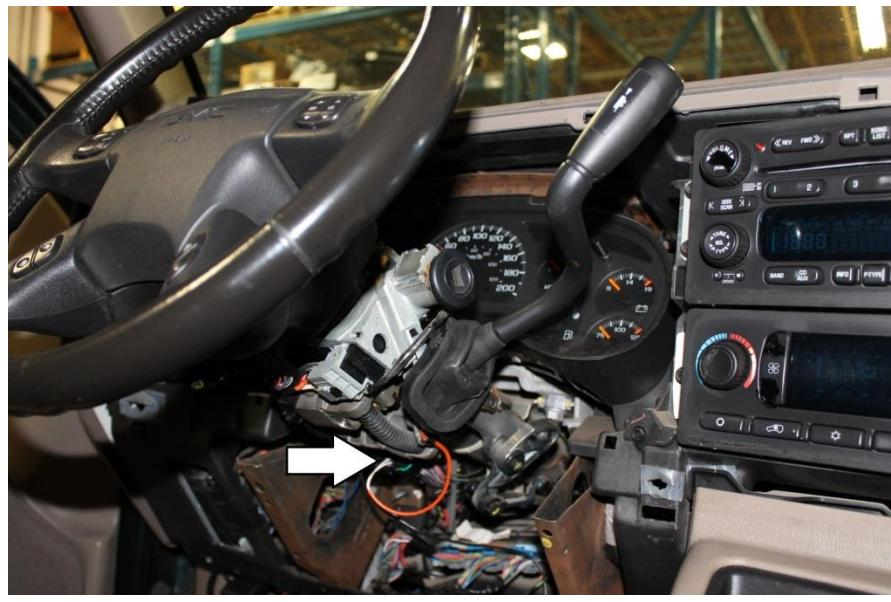
7. Pull back the rubber boot on the shift lever. Using a T27 torx bit, remove the screw attaching the shifter lever to the mechanism in the column.
