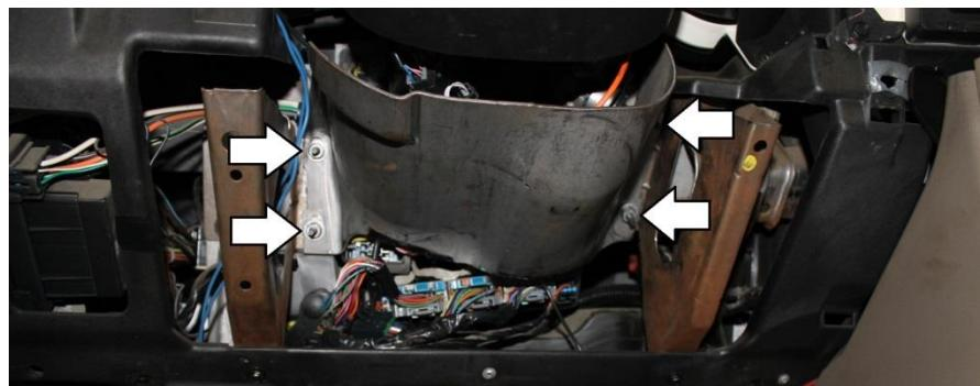
5. Remove the tilt lever from the steering column (1) and the screws from the bottom side (2). Unclip the upper and lower covers. Use care not to break the clips on the covers.
