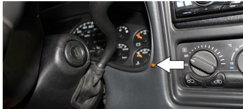
28. Fish the BLACK wire from the LED through the firewall to the TCM at the front of the engine bay.
