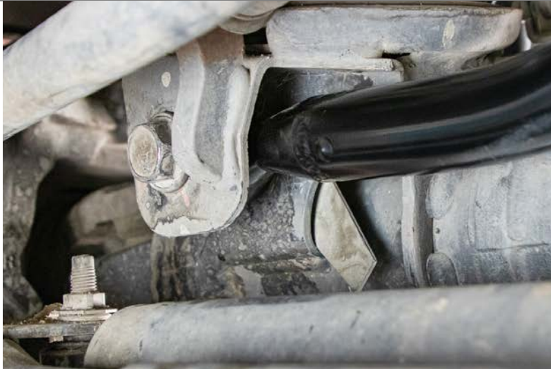
Figure 8: Passenger side nut in position.
