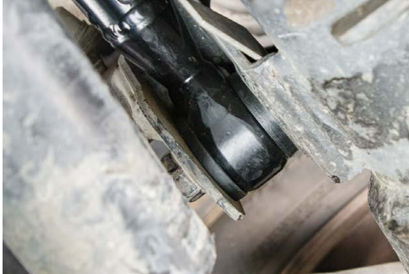
Figure 7: Install the passenger side of the bar with poly bushings.
