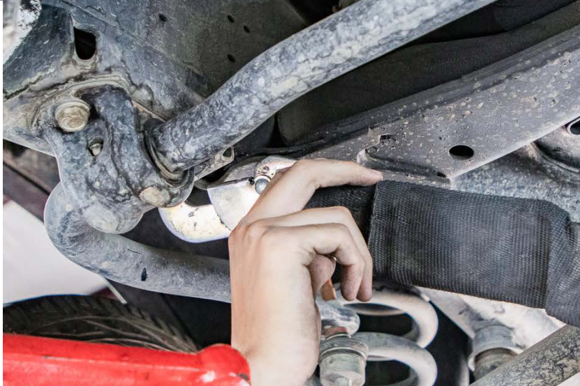
Figure 1: Hook ratchet to the passenger sway bar bracket on the frame.
