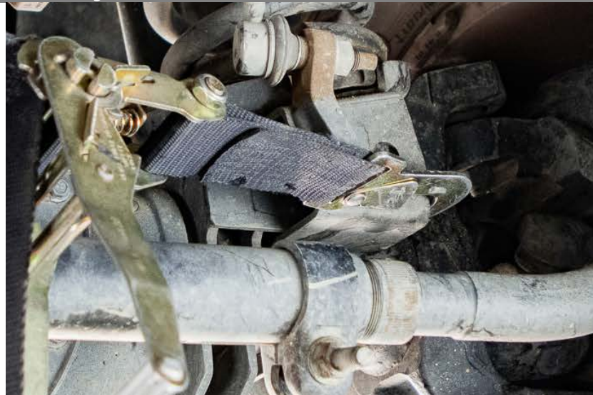
Figure 2: Hook ratchet to the driver end link bracket.
