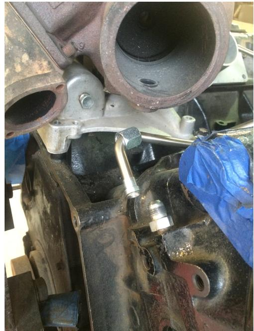
2. Remove factory wiring harness and lay over the the passenger side of the engine bay. This will allow you to get the lines where they need to go to the back ports. The lines will lay just over the top of the heads below the injector harness. You will have to remove the lifting eye on the passenger head and leave it off to route the line properly.
