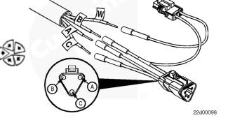
NOTE: The illustration shows the labels of the wires from the rear of the connector.
