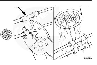
After installing the jumper harness, wrap the excess wires in electrical tape, then route the wires through the convolute's terminating end. Continue to wrap electrical tape around the convolute at least two times. This will make sure the wires do not fall out and short to ground, or chaff against the convolute's sharp edges.
