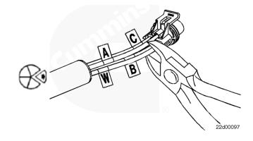
Located on the electrical repair connector are the labels with the correct numbers and letters. Match the labeled wires together.
