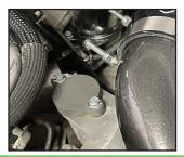
Re-install factory fuel filter cup and all previously removed bolts, tighten all bolts. Re-install upper fuel filter and fuel lines.
