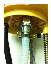
Step 9. Remove OE components from bottom of module basket, remove top screen (fig 10) but leave bottom screen intact. Drill out center hole to at least 5/8" to allow hard Nylon tube to pass through hole.
