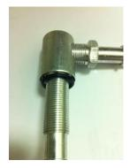
Step 6. Install the washer on the bulkhead fitting first then tighten the Nyloc nut.
