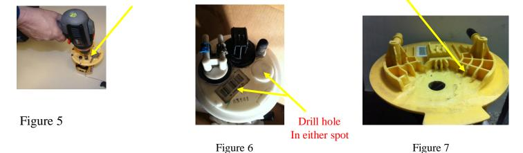
Step 3. Removing pump from module.
