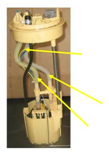
An alternate method is to cut the black plastic supports (there are 3) around the top of the pump that are attached to the basket and remove entire assembly, the end result will look like fig 9. This will expose a small rubber valve at bottom of module (fig 8) that will allow fuel to enter module from below.
