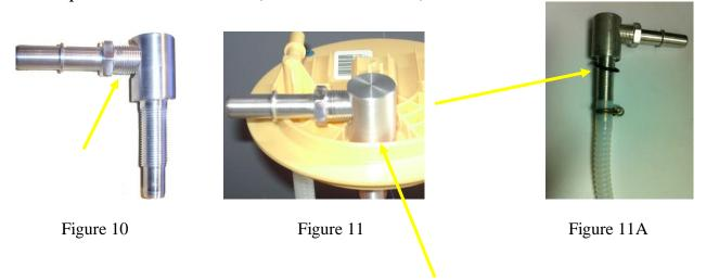
Step 6.Insert the bulkhead fitting with the washer, o-ring side down, into the 5/8" hole.
