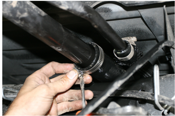
(Fig. 12) Attach fuel tank 1 ½" fill hose and ¾" vent hose to vehicle fill spout. Vent hose may have to be shortened about 6 inches to fit properly. On some long bed tanks, 1 ½" fill hose may have to be extended with 3.35" hose extension.
