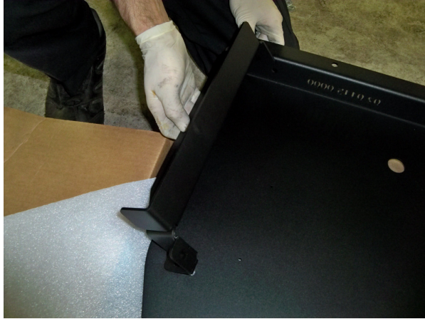
(Fig. 1) The Skid Plate Nose Cradle Bracket attaches to the base of the Skid Plate with two carriage bolts included.
