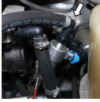
67. Trim fuel tube to length, and secure with 1500387 spring clamp.Tighten banjo bolt to 18 ft-lbs using 3/4in socket.
