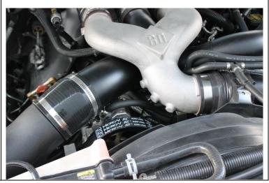
69. Prime fuel system several times using the filter pump, or lift pump and start engine. Check for leaks.
