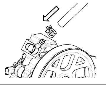
68. Re-install intake tube, and any other components removed for install of pump.
