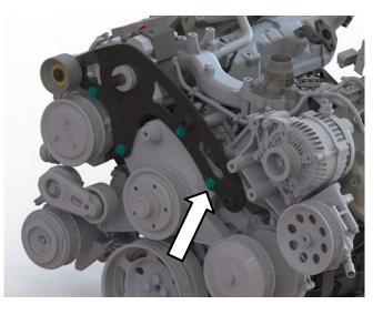
27. Install OEM idler pulleys onto bracket using OEM hardware. Using a 15mm socket, torque fasteners to 35 ft-lbs.
