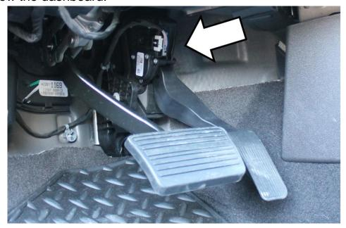
Connect supplied wiring harness to the accelerator pedal position sensor and the
