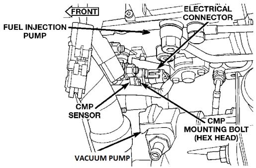
**2003-2004 Dodge 5.9 (CR)** – Locate the engine crankshaft position sensor, located toward the front of the engine on the left side beside the harmonic balancer. Cut off and discard the supplied three pin connector from the blue wire on the BD wiring harness (this is used only up to 2002). Tap the blue wire into the crankshaft sensor wire from pin 3 of the connector. Solder this connection and cover with heat shrink for longevity.
