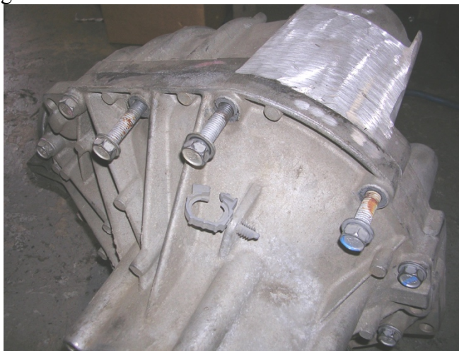
Figure 1: Clean up excess material left from previous mount
