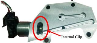
If your pressure sensor doesn't have the internal clip, discard the factory retainer and use the ATS supplied retainer.
