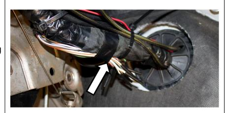
2. Cut the tape holding the wires in place. Identify and separate the appropriate wires for your model year vehicle. (see table below) Some years have a label with this information taped to the harness. Cut the heat shrink tubing off the ends and strip the wires.
