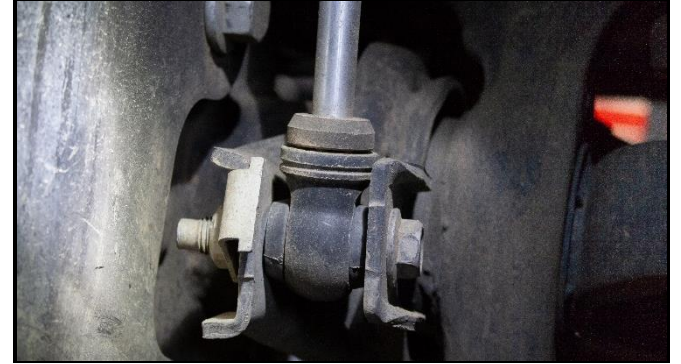
Figure 10: Front Lower Shock Mount Installed
