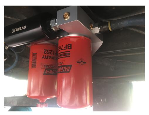
3. Once the supply line is attached to the T fitting in the valley you can now run the new line off of the regulator behind the AC compressor also. This line will attach to the factory return hard line on the frame with supplied quick connect fitting on 3/8" fuel line. The return line is located just behind the drivers side front tire, or below the steering shaft. The top hard line is the return line to be used as pictured below.
