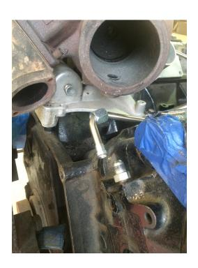
2. Remove factory wiring harness and lay over the the passenger side of the engine bay. This will allow you to get the lines where they need to go to the back ports. The lines will lay just over the top of the heads below the injector harness. You will have to remove the lifting eye on the passenger head and leave it off to route the line properly.
