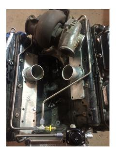
6. Install the 1/8npt x 6 jic  $45^*$  fittings into both the front ports on the head pointing straight up.
