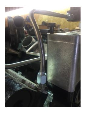
7. With all fittings installed you can now install the back lines and connect them to the supplied #6 jic T fitting in the valley of the motor. This is where you will **supply** fuel to. (See pics for reference)
