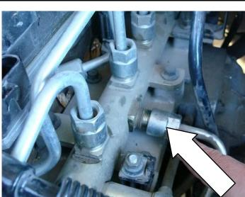
14. Remove the banjo bolt with washer from the front side of the fuel rail (17mm wrench). Careful not to lose the washer when you pull out the banjo bolt.
