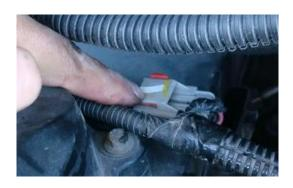
19. Disconnect the EGR servo motor connector.
