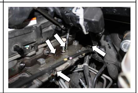
25. With the four bolts removed you may need to gently pry the grid heater from the gasket before it can be removed from the vehicle.
