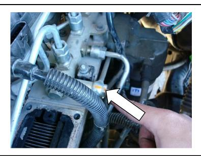
15. Remove the six injector lines starting with the loosening the fittings at the front of the fuel rail and the #1 injector (19mm wrench). (NOTE: Fittings on both sides of the line will need to be backed off before the line can be removed).
