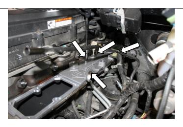
Reconnect the fuel rail connector. Then apply some pipe dope to the four OEM fuel rail bolts and reinstall the fuel rail to the intake plate. Torque to 18 ft/lbs. (10mm socket)
