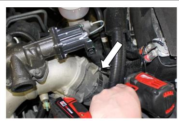
7. Pull off the harness clip from the intake horn.
