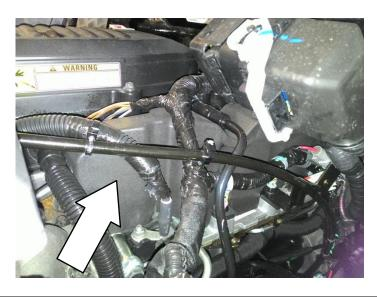
13. Loosen the fittings on the line that goes from the fuel rail to the CP3 pump, once both fittings are loose the line can be removed from the vehicle. (19mm Wrench)
