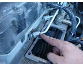
16. Disconnect the Intake air temperature sensor connector from the grid heater.
