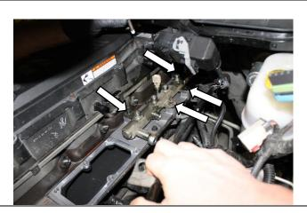
Reinstall the six injector lines (19mm wrench) an easy task if marked for identification, not fun if not.
